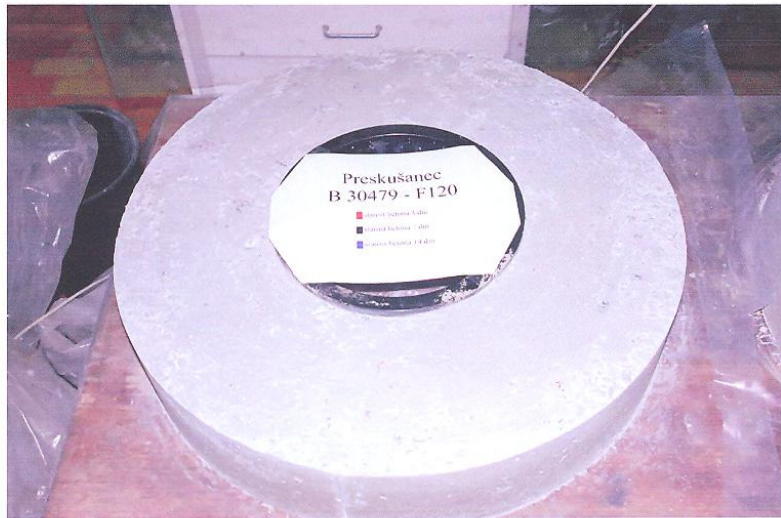
Picture 4: Concrete with fibres FIBRILs F120 – 0.95 kg / m 3
