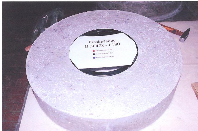
Picture 3: Concrete with fibres FIBRILs F180 – 0.95 kg / m 3
